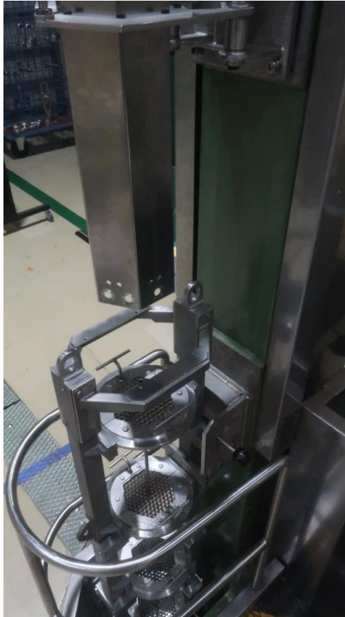
Fig 5. Shroud and Fuel Assembly assembling station.
