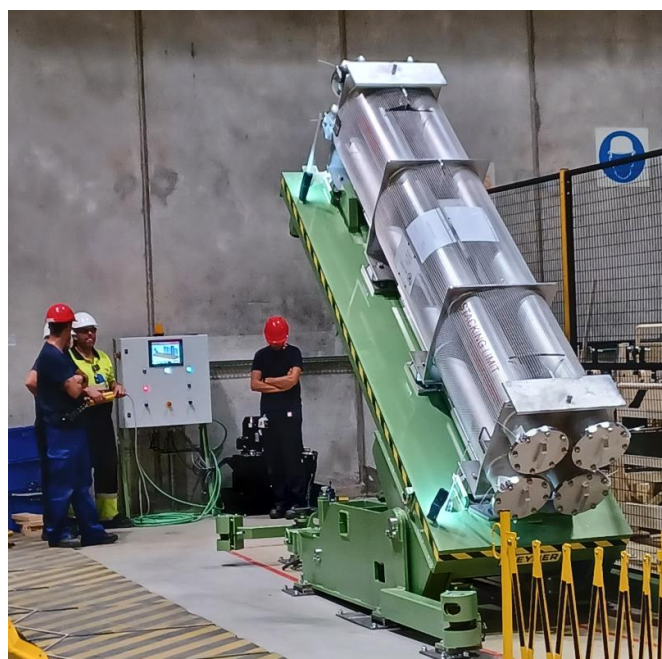
Fig 6. Tilt equipment for fuel packaging
