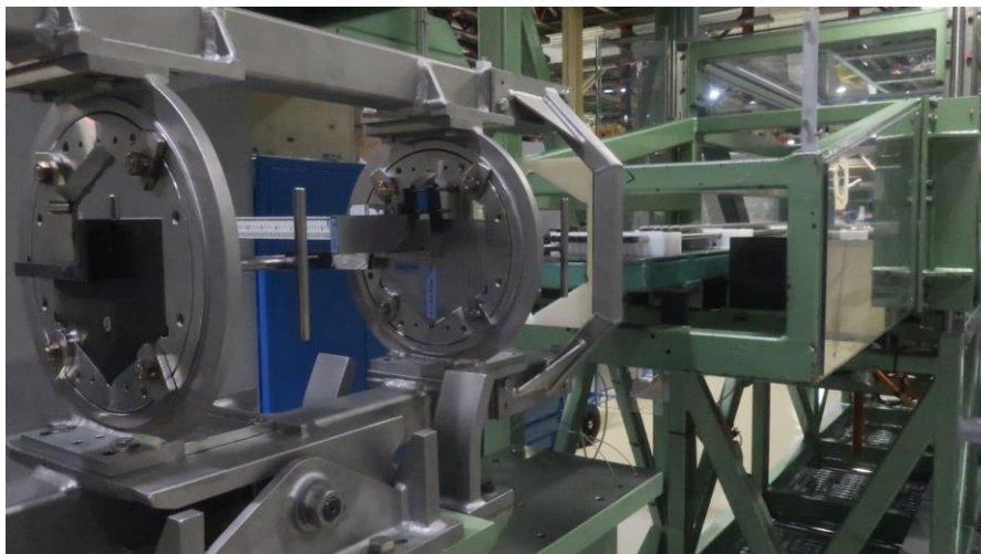
Fig 4. Fuel rod loading into the skeleton equipment
